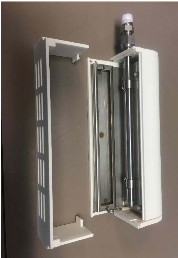
Figure 11c. The bar with cover removed to show how the sources are loaded
