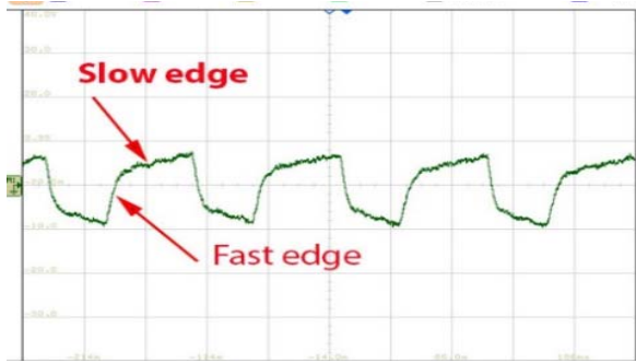
Figure 4. Hybrid alpha ionizer with square wave. Note the taller fast edge compared to Figure 3.
