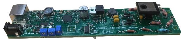
Figure 11a. The circuit board is clean owing to the use of the microprocessor.
