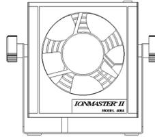
The Model 4064 Ionmaster™ II Fan is used to create airflow through the Ionizer (model P-2063 Nuclecel™). This system delivers a high volume of ionized air to reduce charge on parts. The Fan is mounted on a swivel base and can be placed on a flat surface or bolted to a rigid surface.
